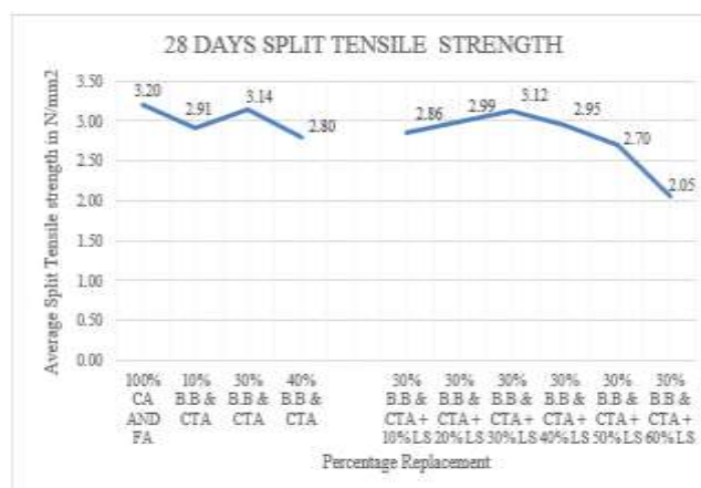
Chart -11: Split tensile strength test results for 28 days
