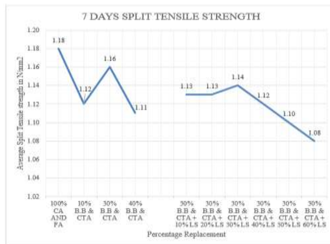
Chart -9: Split tensile strength test results for 7 days
