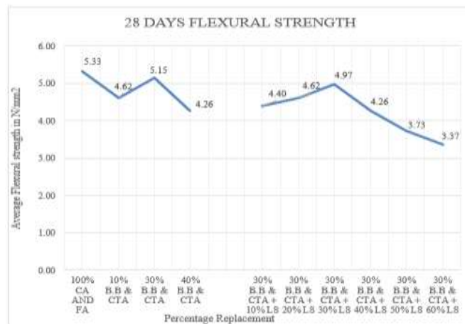
Chart -8: Flexural strength test results for 28 days
