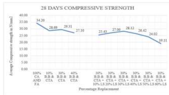
Chart -4: Compressive strength test results for 28 days
