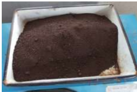
Fig- 2: Lead slag in form of fine aggregate
