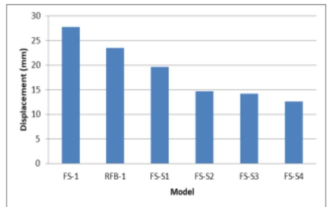
**Graph-1: Variation of roof displacement by equivalent static analysis for G+ 3 structures.**
