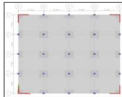
**FS-S1- Flat Slab Building with Shear wall at exterior corner location.**
