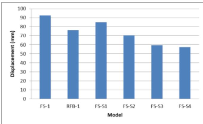
Graph-2: Variation of roof displacement by equivalent static analysis for G+ 9 structures.
