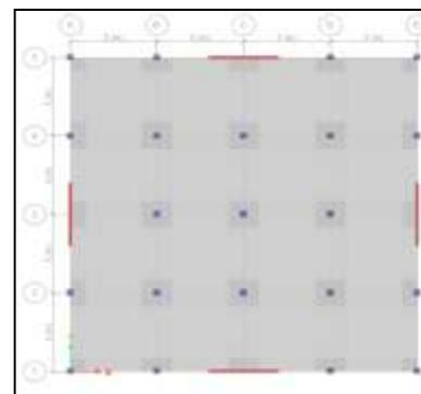
**FS-S2- Flat Slab Building with Shear wall at exterior mid location.**
