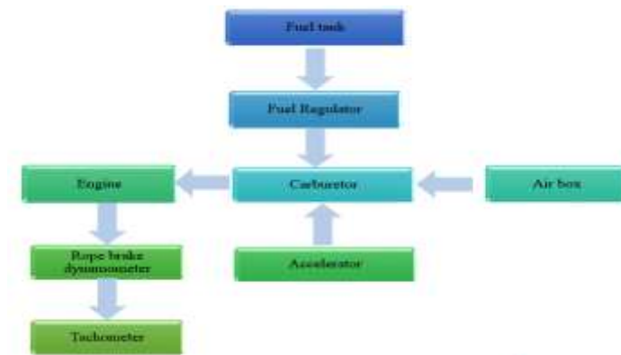
Fig -1: Schematic diagram of the Test Rig
