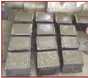
Fig.3: Casting of Cubes
