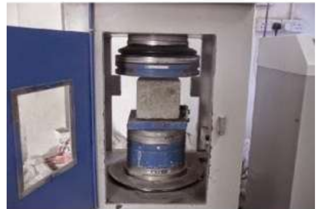
Fig.4: Compressive Strength Testing Machine
