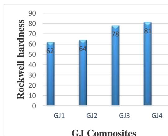
Fig-5. Rockwell Hardness of tested Specimen
