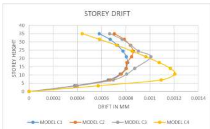
Fig -4.2: Storey drift of Structure
