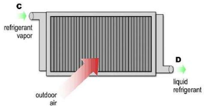
Fig -3: Basic Condenser System
