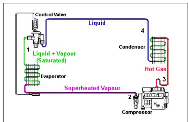
Fig. 1. Basic Refrigeration System
