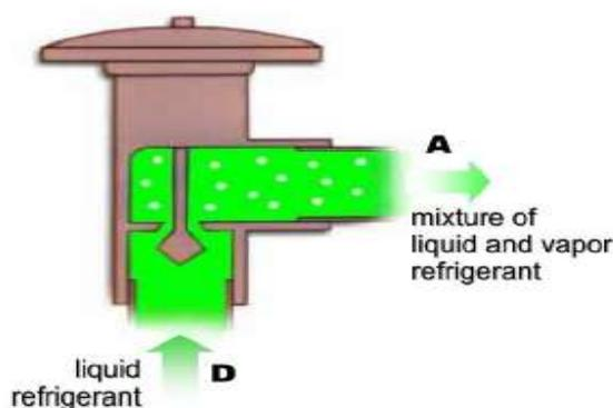
Fig -5: Basic Expansion Device System
