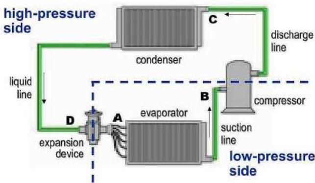
Fig -6: Basic Vapour Compression Refrigeration
