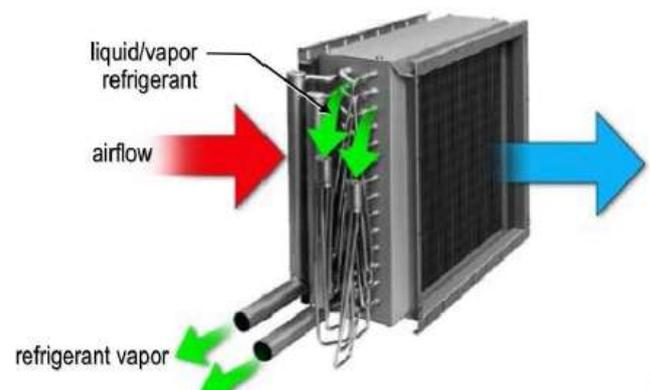
Fig -4: Basic Evaporator System
