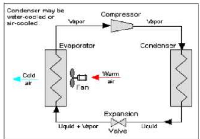
Fig -6: Schematic Vapour Compression Refrigeration
