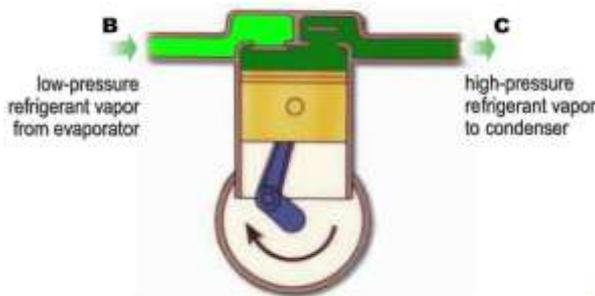
Fig -2: Basic Compressor System
