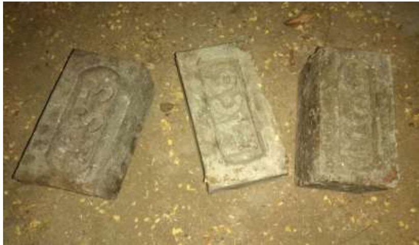
Figure 1 - Sample of casted Hypo-Sludge Bricks.
