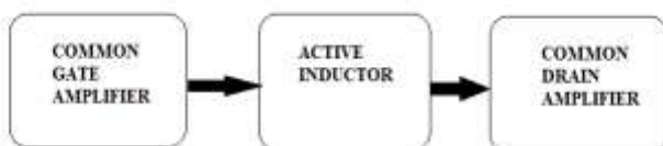
Fig -1: Block diagram of the proposed LNA [1].
