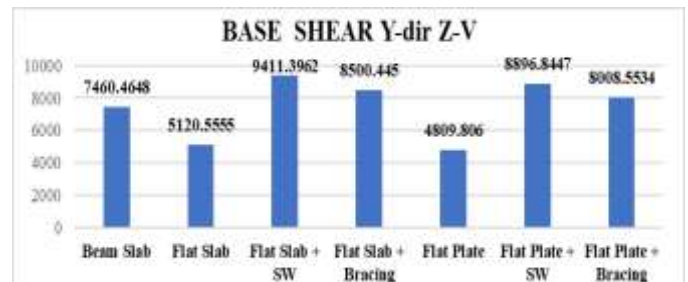
Fig 17. Base Shear(kN) along Y-direction in zone-V
