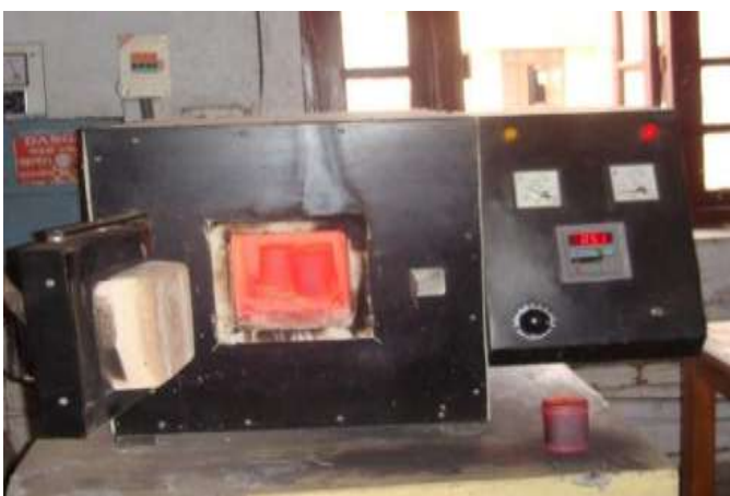
Fig -4(B): Muffle furnace for carburization
