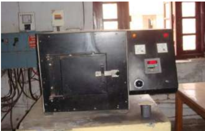
Fig -4(A): Muffle furnace
