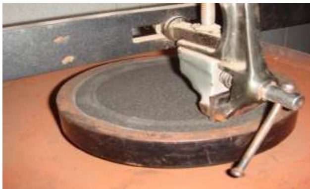
Fig -5(B): Pin on disc machine for abrasive wear testing
