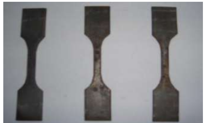
Fig -3(A): Specimen for tensile test
