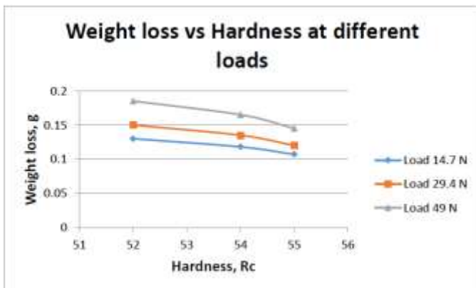
Chart -17: Comparison of weight loss due to abrasion VS hardness for the three Different loads of 14.7 N, 29.4 N and 49 N
