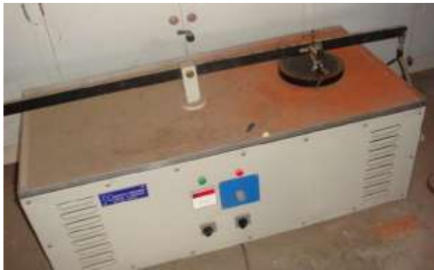
Fig -5(A): Pin on disc machine for abrasive wear testing
