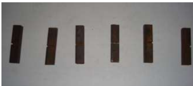
Fig -2(B): Specimen for toughness test
