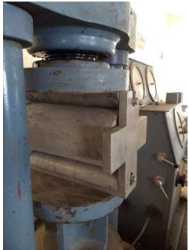
Fig 2. Split tensile strength test
