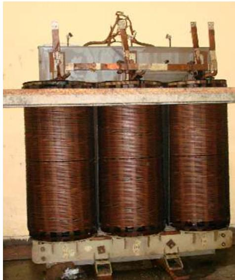
Fig. 1 Core assembly out of tank
