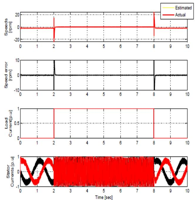
**Fig -12:** Simulation results of sensorless speed control with load change ( $T_L = 0$ ) at zero speed.
