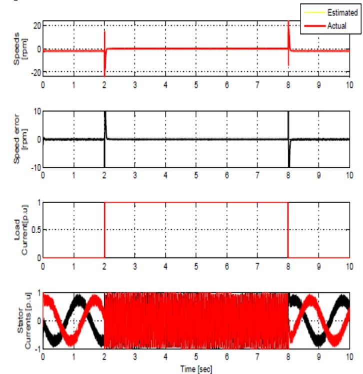
Fig-8: Simulation results of sensorless speed control with load change ( $T_L = 0 \rightarrow$  rated torque  $\rightarrow 0$ ) at very low speed of 2 rpm.
