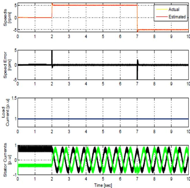
**Fig -14:** Simulation results of sensorless speed control with rated load torque at step speed change and speed reversal at 5 rpm.
