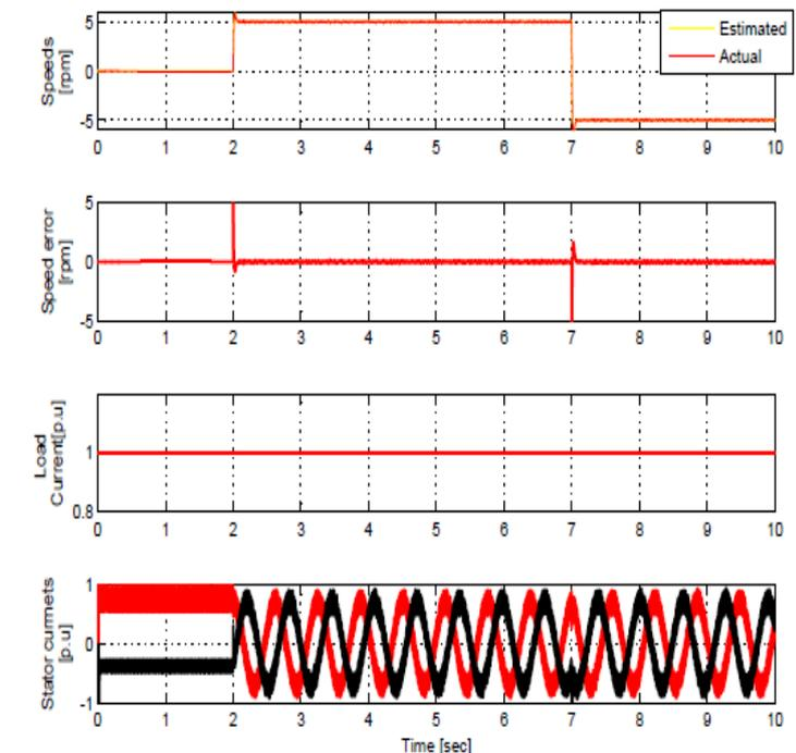
Fig.-9: Simulation results of sensorless speed control with rated load torque at step speed change and speed reversal at 5 rpm.
