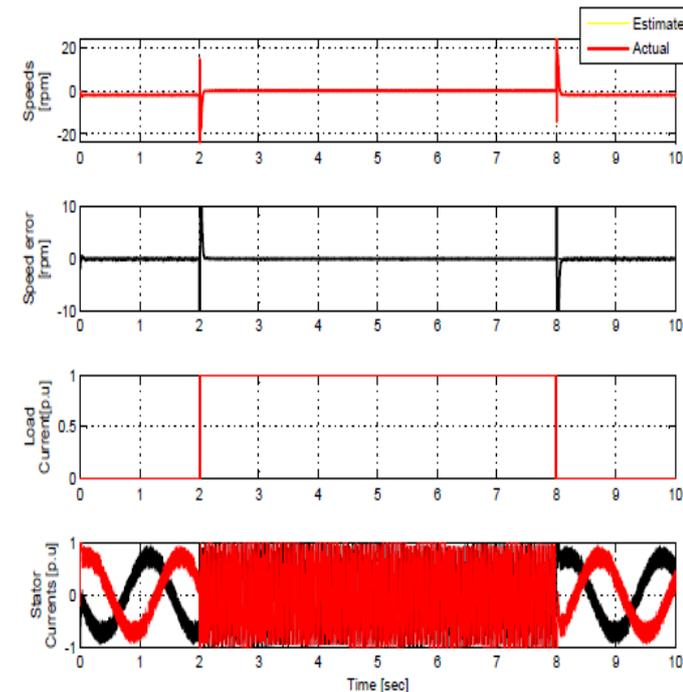
Fig -7: Simulation results of sensorless speed control with Load change ( $T_L = 0$ ) at zero speed.
