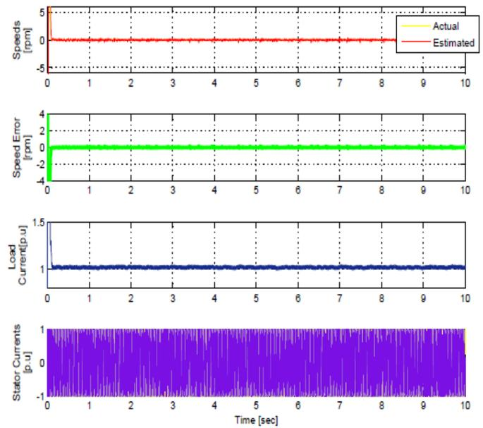
**Fig-11:** Simulation results of sensorless speed control with Rated load torque at zero speed.
