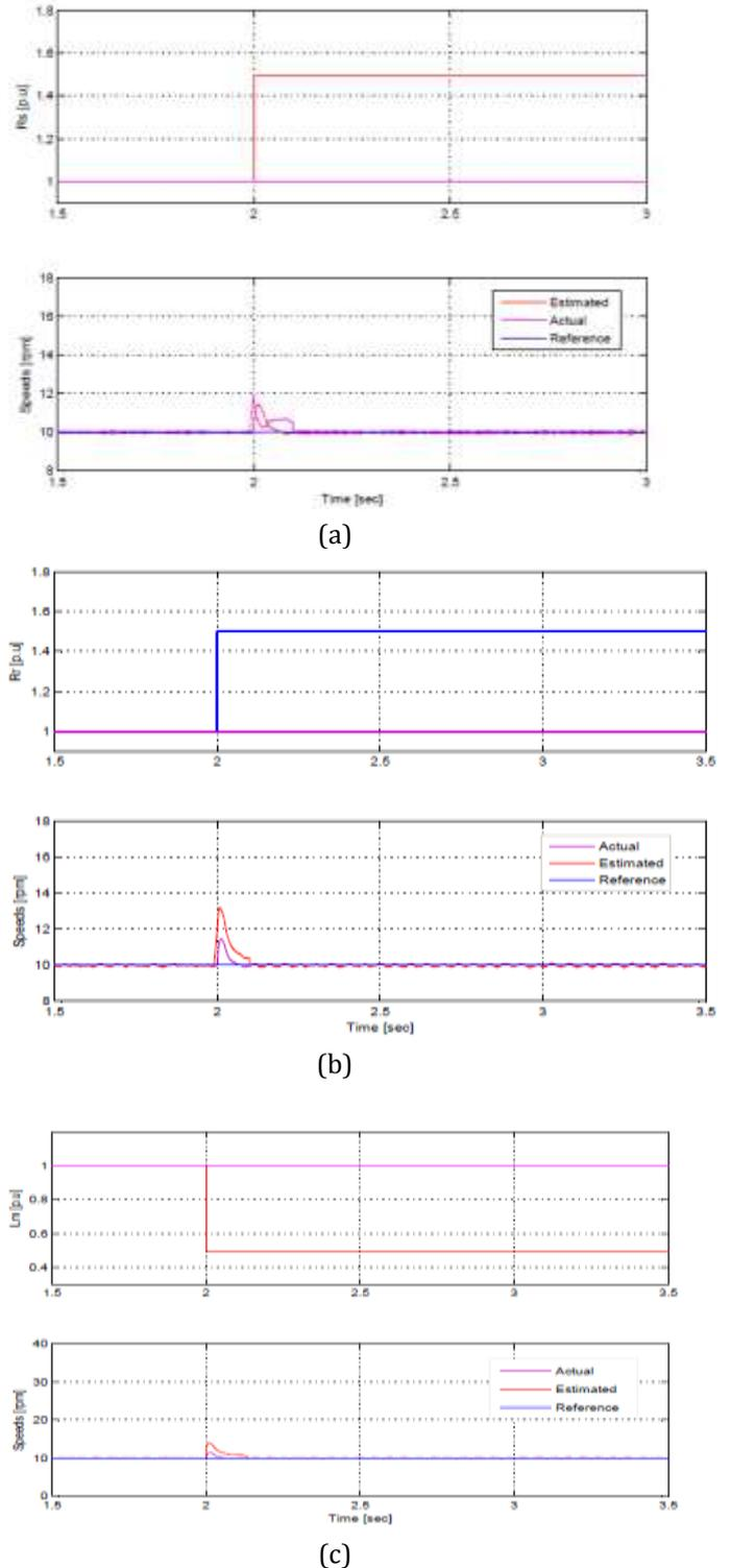
**Fig -15:** Simulation results showing the performance of the proposed SMO under the effect of parameters variation during low speed of 10 rpm and rated load torque. (a) 50% step change of stator resistance. (b) 50% step change of rotor resistance. (c) 50% step change of mutual inductance.
