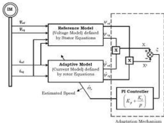
Fig-2: Block diagram of speed estimation using MRAS
