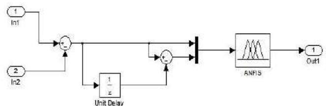
Fig-5: ANFIS controller in proposed system Rules are fired and one output by system
