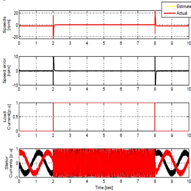
**Fig-13:** Simulation results of sensorless speed control with load change ( $T_L = 0$ ) at very low speed of 2 rpm
