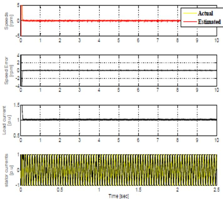
Fig -6: Simulation results of sensorless speed control with rated load torque at zero speed.
