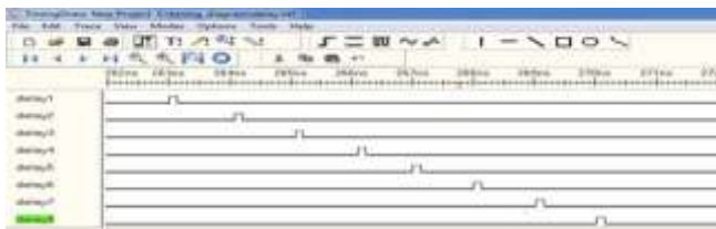
Fig. 2. Signal flow through delay line
