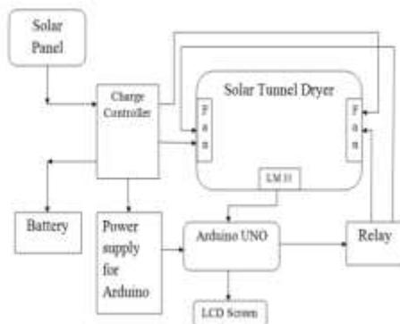
Fig. 2: Block diagram of solar tunnel dryer
