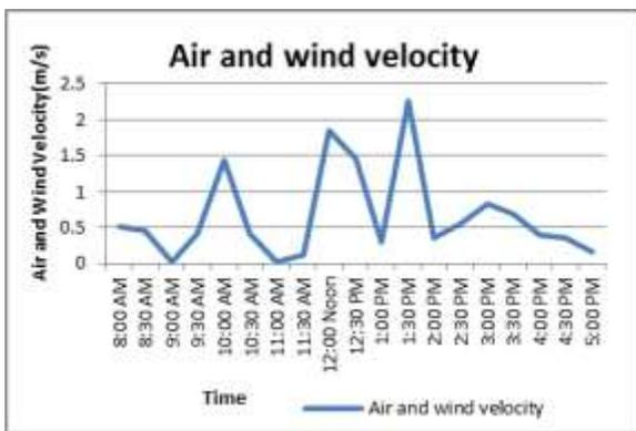
Fig. 6: Variation of air flow velocity with time at no load condition
