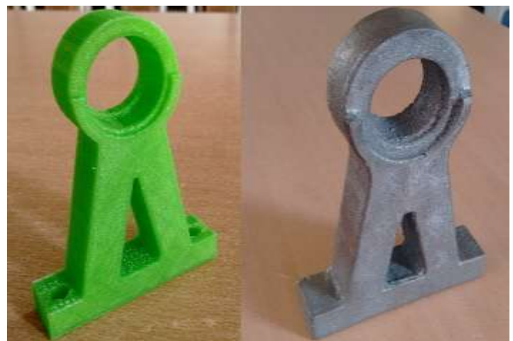
Fig -7: RP model and Final Casting manufactured.
