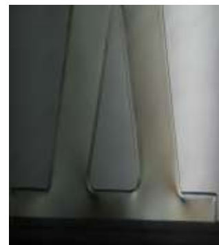
Fig -6: Experimental test on photoelastic model of optimized roller bracket on polariscope.
