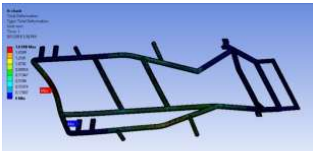
Fig- 17: REAR IMPACT, DEFORMATION
