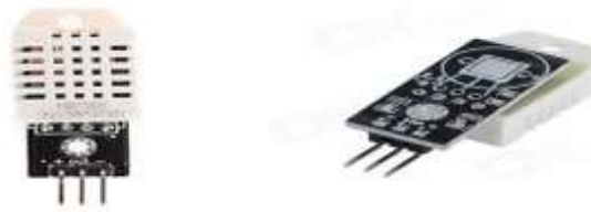
Fig.-7:DHT22 Sensor Module
