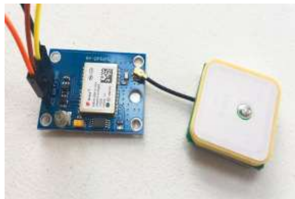
Fig.-11: GPS module with antenna connected
