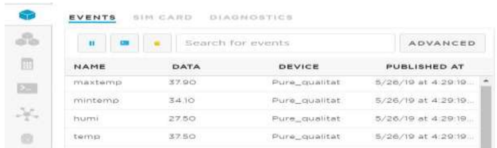
Fig-18: Slave 1 DHT22 Sensor Readings on Particle Cloud That Is Temperature, Humidity, Minimum And Maximum Temperature.
