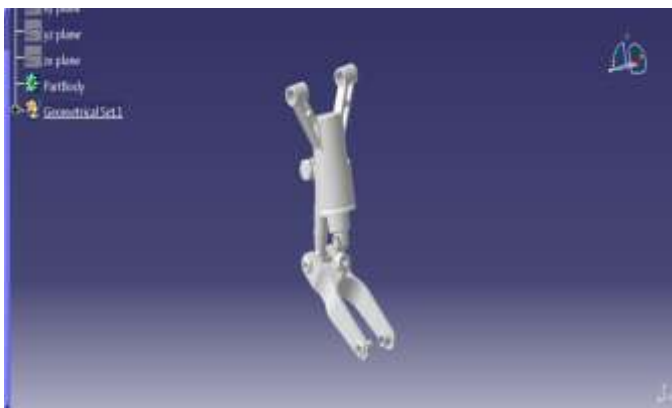
Figure no 2: 3d view of Landing gear
