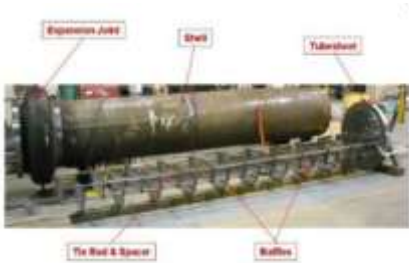
Fig.1.Components of Shell and Tube Heat Exchanger
