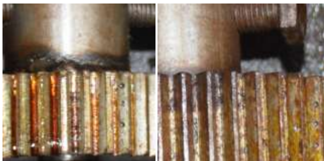
Fig5. Slight pitting on gear and pinion
