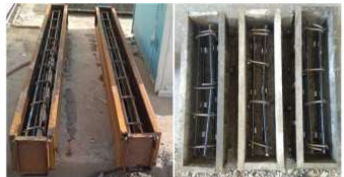
Fig -2: Beam specimen Used for casting(Steel & Bamboo)
