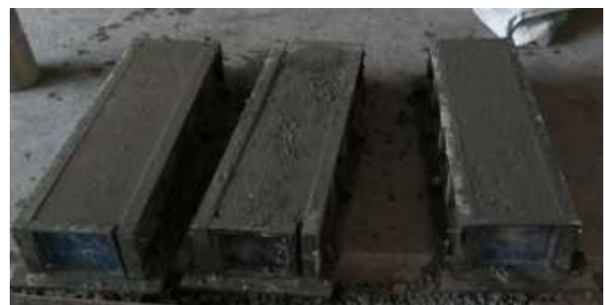
Fig -3: Beam specimen after casting
