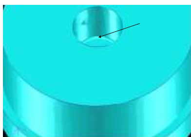
Fig 2.1.1a Design modification with 2 mm fillet radius
