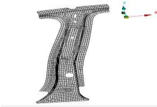
Fig 3.4 Meshed FE Model of B-pillar
