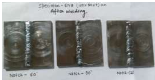
FIG 2.2-WELDING OF EN8 PLATE
