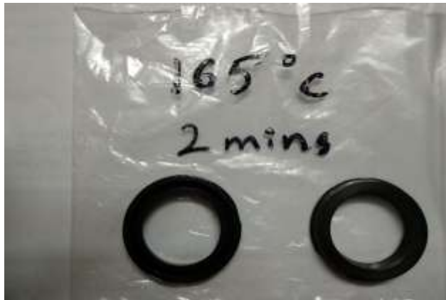
Fig-9: Nut ring samples at 165°C and 2 minutes of curing time
