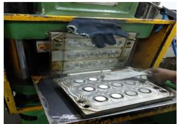
Fig-7: Final assembly of mold die
