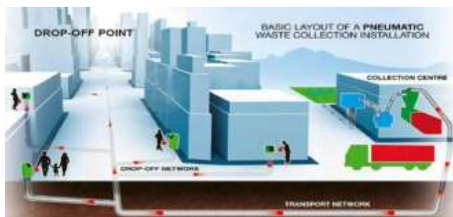
Fig -5: Pneumatic Waste Collection System
