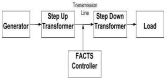
Fig -6: Block diagram of compensation scheme
