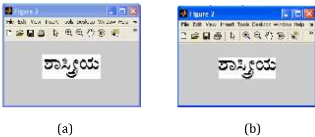
Fig 4.2.3: a) Binarized Image before Boundary Box Fitting b) After Boundary Box Fitting
