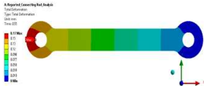
Fig.8a Total Deformation of connecting rod
