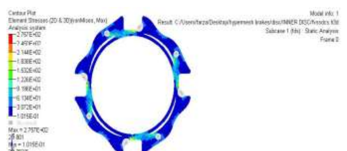
Figure- Elemental Stress Result of Inner Disc
