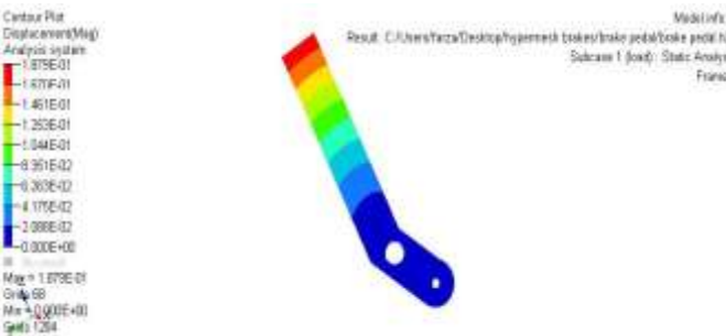
Figure- Displacement Result of Brake Pedal
