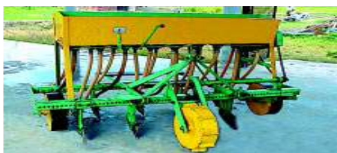
Zero-till seed-cum-fertilizer drill mechanism
