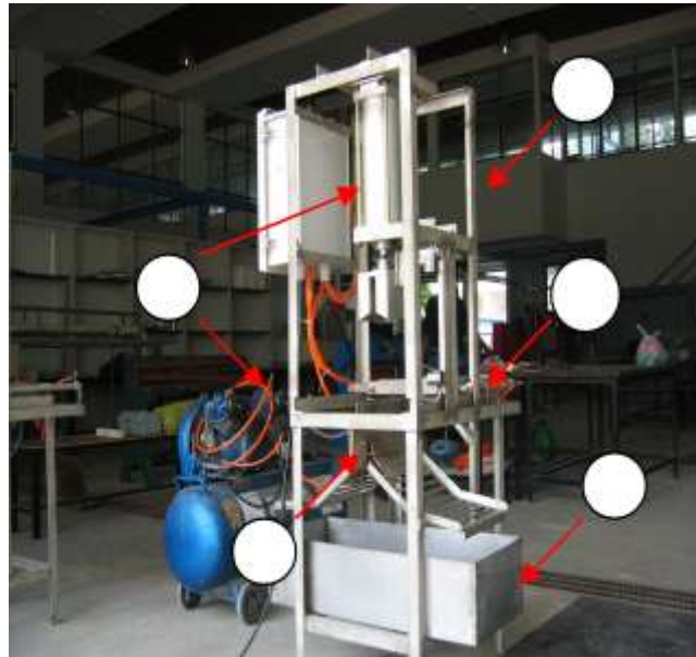
Figure 4. Prototype of the semi-automatic young coconut fruit cutting machine: 1) machine frame; 2) cutting base; 3) knife set; 4) pneumatic system; 5) tank
