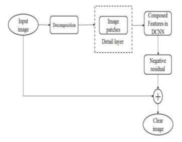
Figure 1: Rain streaks removal system architecture
