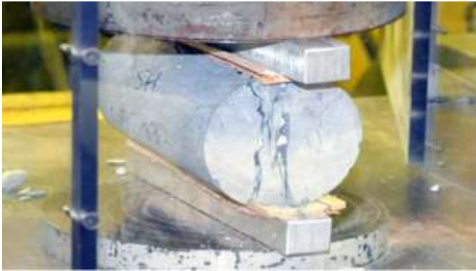
Figure-3: Split Tensile Strength Set
