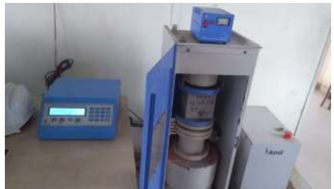
Figure-2: Compressive Testing Machine Set
