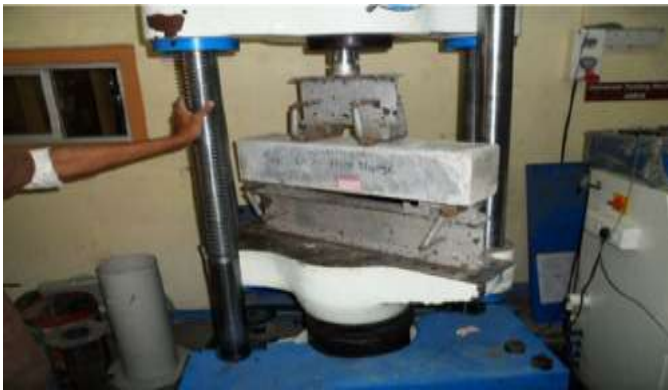
Figure-4: Flexural Strength testing set at UTM
