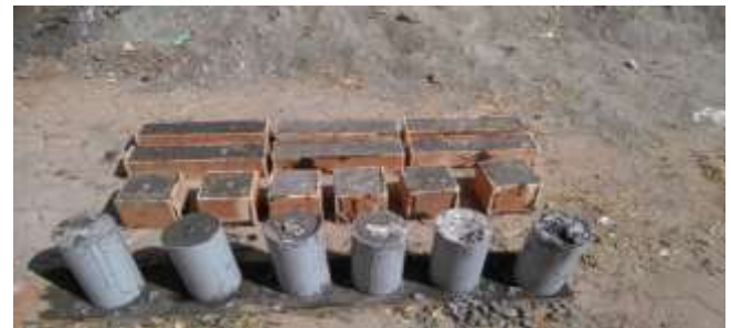
Fig-1 Casting of Geopolymer concrete
