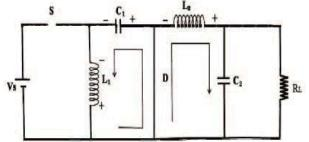
Fig. 9 mode 1 operation of zeta converter
