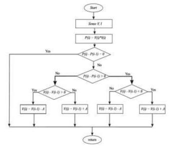
Fig. 2 Flowchart of P & O algorithm
