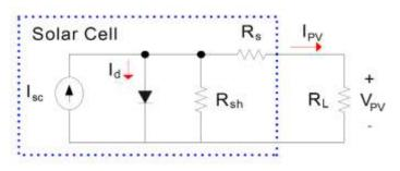
Fig. 1 equivalent circuit single diode model
