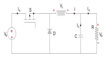
Fig. 3 Buck converter
