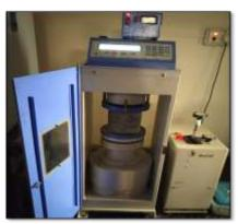
**Figure 1.2** shows the testing of concrete cube specimen in compression testing machine
