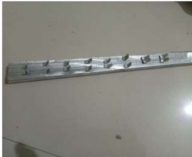
Fig.20. Alluminum Plate with vortex generator in inline arrangement.
