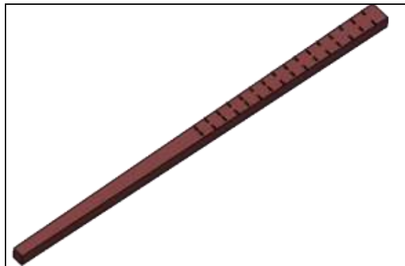
Fig.3.shows staggered arrangement of semi-circular vortex generator.
