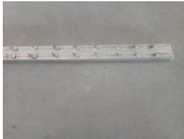
Fig.19. Alluminum Plate with vortex generator in inline arrangement.
