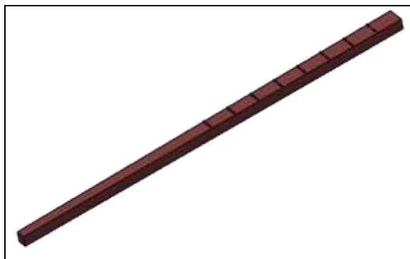
Fig.2. shows Inline arrangement of semi-circular vortex generator.
