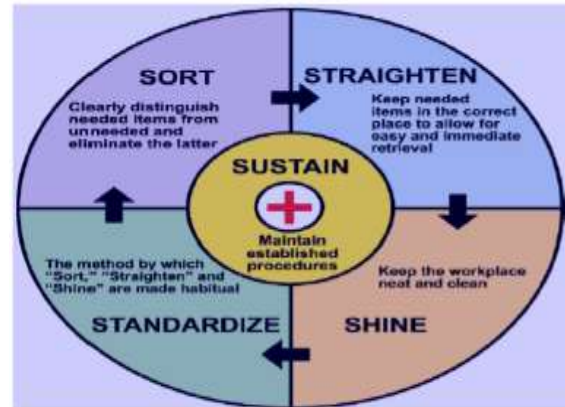
Figure 4: The Schematic Diagram of 5S principles
