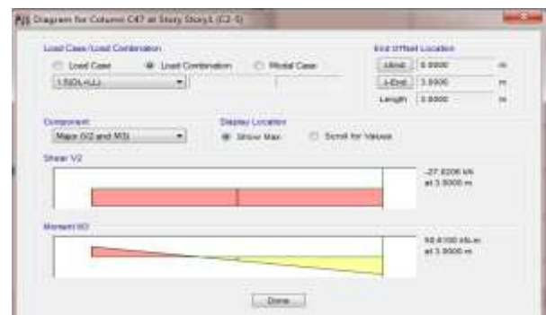
Fig-8 : Bending Moment and Shear force diagram of column C47
