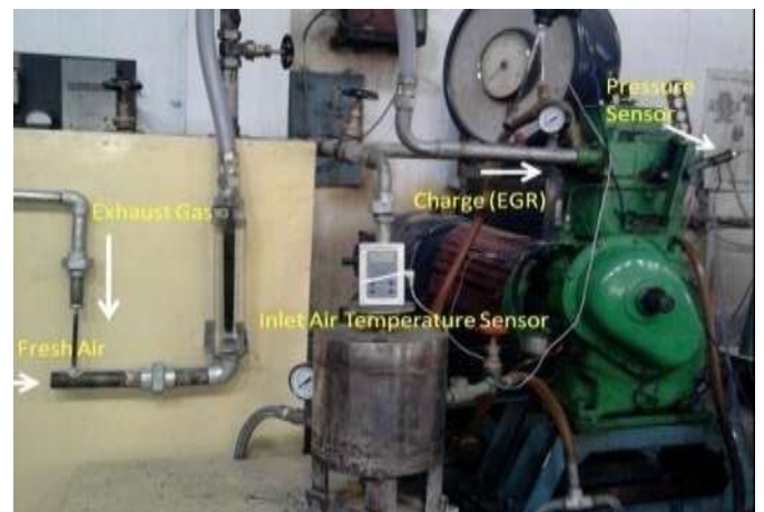
Figure 3.6: Photographic view of experimental setup showing EGR path
