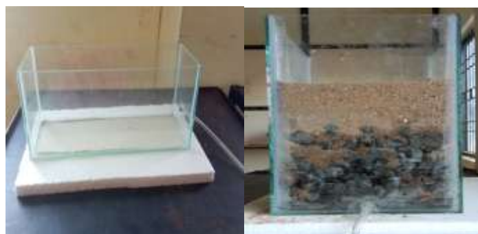
Fig-2 : Sedimentation tank & Filtration tank
