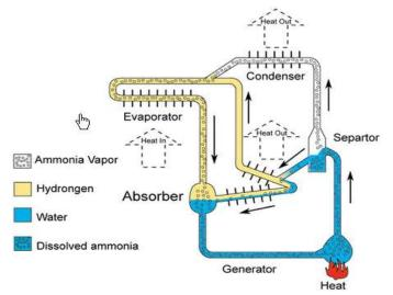
**Fig-2:** Three fluids (Ammonia-Water-Hydrogen) vapour absorption refrigeration system
