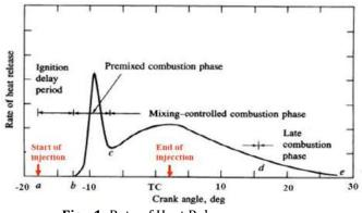
**Fig - 1:** Rate of Heat Release curve
