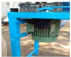
**Figure 5.2 d:** Connection of motor shaft to shake table frame
