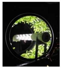
Fig. 4.2.1 rotary hydroponics system
