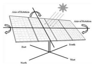
Figure 1 – Representation of a Solar Tracker
