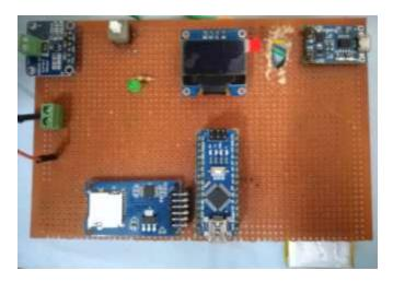
Figure 3 - Representation of Digital Portable Data Meter and Logger
