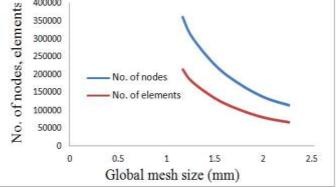
Figure 6. Mesh size versus number of nodes and elements
