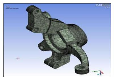
Figure 4. Unstructured mesh of knuckle using Tet10 elements
