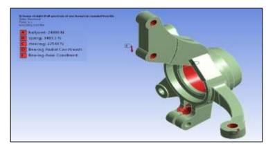
Figure 3. Location of applied loads and constraints
