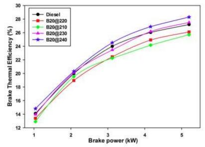
Fig. 3 Variations of brake thermal efficiency with brake power
