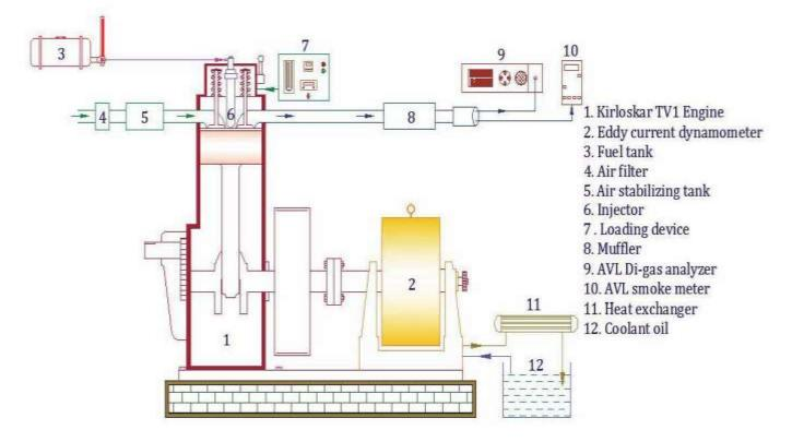
Fig. 2 Experimental setup (Kirloskar TV-1 Engine)
