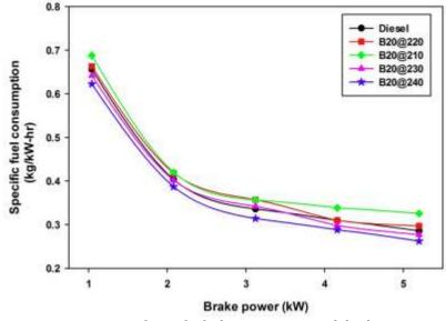
Fig. 4 Variations of specific fuel consumption with brake power
