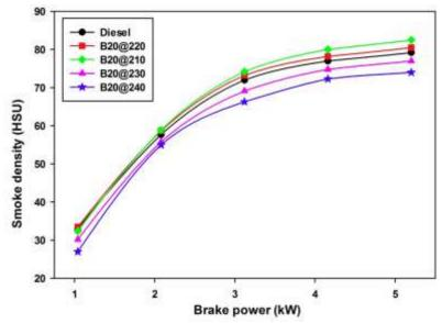
Fig. 5. Variations of smoke emission with brake power
