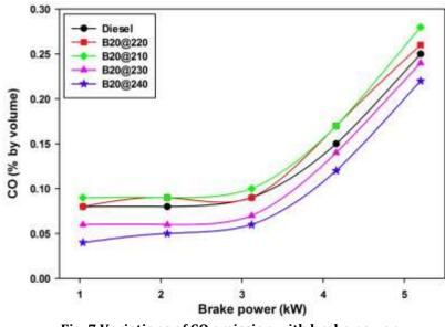
Fig. 7 Variations of CO emission with brake power
