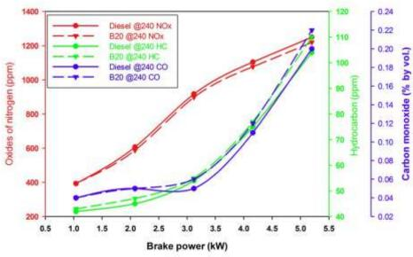
Fig. 9 Comparison of CO, HC and NOx emission
